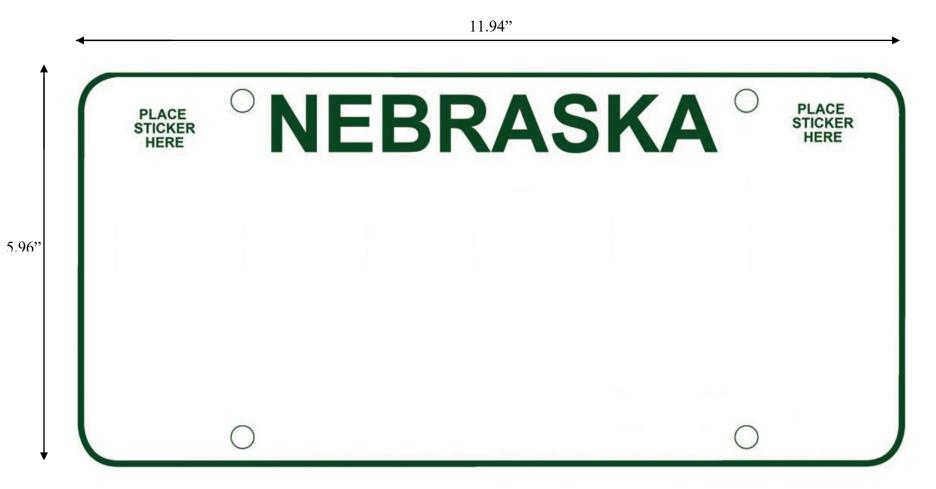
The actual plate size is  $11.94^{\circ} \times 5.96^{\circ}$  with a  $3/10^{\circ}$  rim around the edge of the plate where no printing can occur. Two locations, at the top right-hand corner and top-left hand corner, are reserved for the placement of validation and tonnage decals. Decals are  $1\frac{1}{2}^{\circ} \times 1^{\circ}$  in size.
